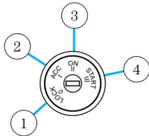
2. If the temperature is above  $-12^{\circ}\text{C}$  ( $10^{\circ}\text{F}$ ) and the engine does not start within five seconds on the first try, turn the key to OFF, wait ten seconds and try again.
