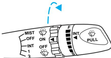
For rear washer fluid operation, rotate the rear wiper/washer control to the desired position.
