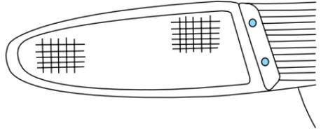
1. Open trunk to expose the tail lamp assembly. Remove the two screws from the front of the lamp.
