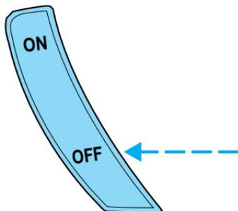
Once speed control is switched off, the previously programmed set speed will be erased.
