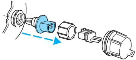
7. Install the new bulb in lamp assembly by pushing straight in with the bulb's plastic base facing upward. Turn the bulb slightly to align the grooves in the plastic base with the tabs in the lamp assembly.
