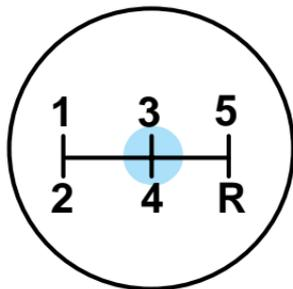
You can shift into R (Reverse) only by moving the gearshift from left of 3 (Third) and 4 (Fourth) gears before you shift into R (Reverse). This is a special lockout feature which prevents you from shifting into R (Reverse) when you downshift from 5 (Fifth).
