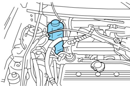
Check the washer fluid whenever you stop for fuel. The reservoir is highlighted with a
