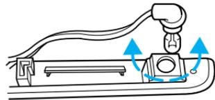
To install the brakelamp bulb:
